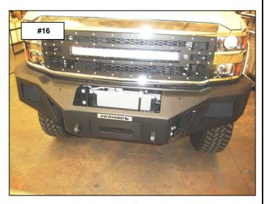
If installing a winch, install the roller fairlead to the bumper shell at this time. Refer to the winch manufacturer's instructions for installation. If installing an optional light bar, install the light bar to the bumper replacement at this time. Refer to the light bar instructions for installation.
