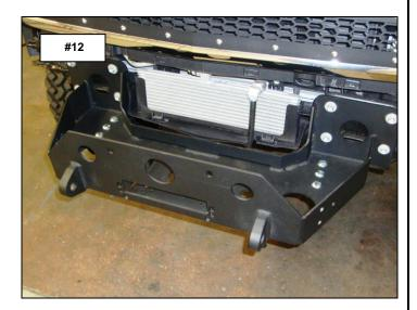
If you are installing a winch, place the winch in the winch tray and refer to the winch manufacturer's instructions for installation. Do not install the fairlead at this time.
