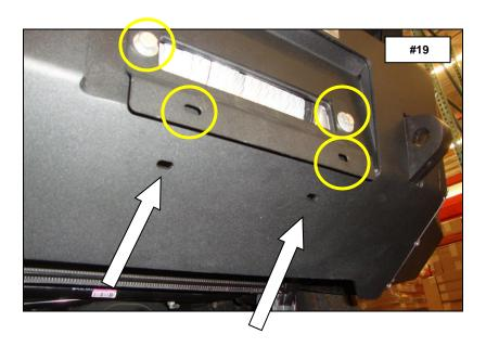
If installing a winch, attach the license plate directly to the (2) obround holes in the lower face of the bumper shell using the supplied 1/4" bolts and nuts, (Photo 18).
