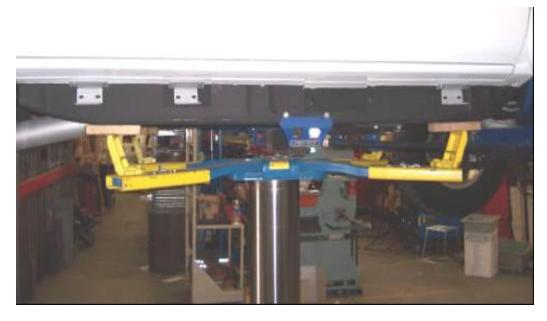
**STEP-5** Position the passenger sidestep up to the mounting brackets and loosely attach it to the brackets using the 3/8" x 1 1/4" hex bolts, (4) flat washers, (2) lock washers and (2) nuts. Align sidestep with the body and then tighten all mounting bracket and sidestep nuts and bolts. Repeat the above installation steps to install the driver side mounting brackets and side step.
