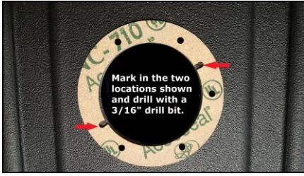
Figure 1: Gasket being used as template to mark drilling locations
