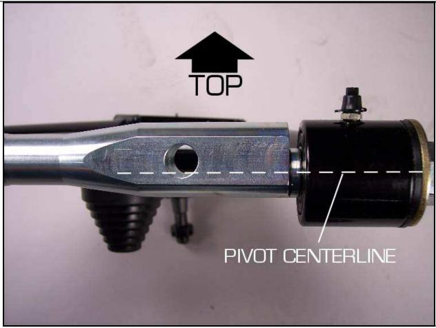
Install the cross shaft onto the vehicle first, using the same nuts that held in the stock arms.
