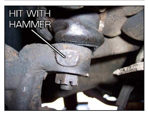
Once the ball joint is loose from the spindle, support the lower control arm with a floor jack and raise the suspension slightly to relieve the pressure on the castle nut. Remove the castle nut and lower the floor jack until the upper ball joint stud comes out of the spindle. You may want to use bungee cords to hold the spindle assembly close to the frame rails as to not stretch/damage the brake lines.
