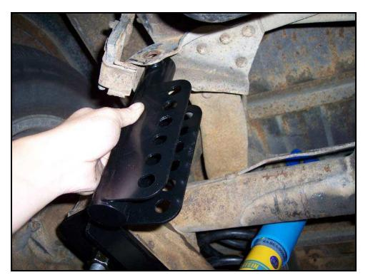
Take the <u>shorter</u> adjustable bar and install it on the  $2^{nd}$  or  $3^{rd}$  hole on the driver side mount bracket. Grease bushing surface with provided lube.
