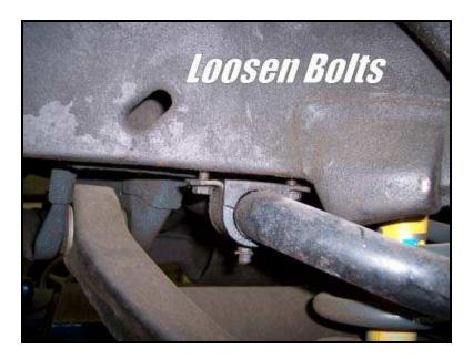
4F. Remove the endlinks from the sway bar and lower control arms.
