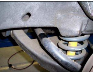
6F. Turn the steering all the way to the LEFT and remove the stock bar through the DRIVER side wheel well. Observe the following pictures for the removal procedure.
