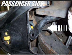
At this point the sway bar will need a little force to get into position. Take your trusty dead blow hammer and hit the anti-roll bar end as shown in the picture below. It won't take too much to pop it into place.
