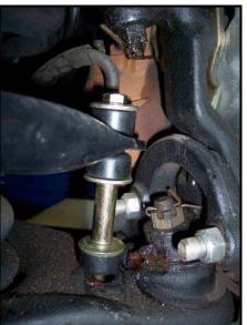
9F. Using the included white silicon grease, lube the inside of the new 1 ¼ " front bushings. NOTE: the grease can be cleaned up with WD-40
