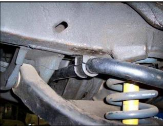
11F. Place the greasable bracket over top the bushing and secure them with the stock bolts. You may fully tighten these bolts at this time.
