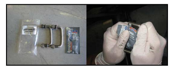
Feed one end of the U-Bolt through one of the holes on either end of the chassis brace and maneuver it into the backside of the other hole as shown below.
