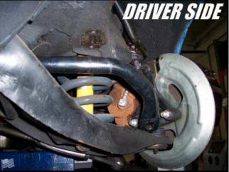
8F. Once the bar is in place, install the new endlinks but do not tighten them completely.
