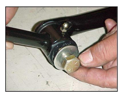
17R. Slide the other end of the dog bone style end link up in between the brackets on the chassis brace. Check for exhaust clearance in this area. If necessary, you may have to have the exhaust pipes re-bent to provide clearance for the new sway bar assembly. Any competent exhaust shop can handle this modification easily. If clear, use the shorter (2.75") bolt with a small washer on each side of the bracket to complete the assembly and fully tighten.
