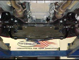
7) Install the subframe mounts back onto the vehicle. Fully tighten all hardware at this time (including the endlink bolts!)
