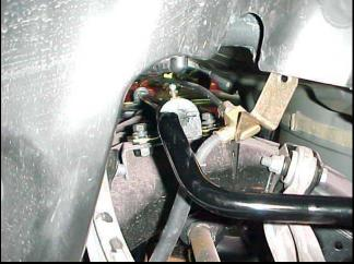
14) Reattach the endlinks to the sway bar in the same manner as removal. Fully tighten all hardware
