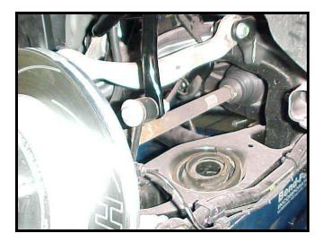
Once everything is in place, raise the rear axle into position. Do not raise all the way up! You will still need some wiggle room to line up the cradle bolt holes. Start each bolt by hand to ensure proper threading. Once thread started, fully tighten the cradle bolts using a 18mm socket.
