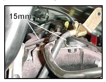
11) The bar should be free to come out. The only obstacle when removing the sway bar is the brake lines may be in the way. If so, carefully push the bar around the brake lines.
