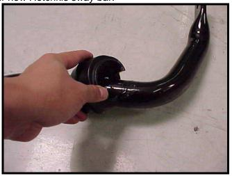
6) Reinstall in the same manner as removal. Attach the endlinks to the sway bar. Do not tighten at this time
