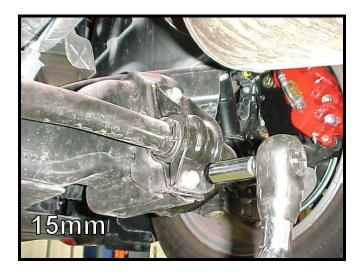
4) Detach the endlinks from the sway bar using a 21mm wrench and a 10mm wrench.
