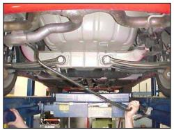
4.) Now your ready to grease the new bushing with the provided grease. Then place the bushing over the bar followed by the bracket.
