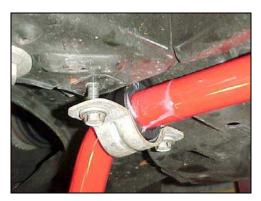
5.) Now install the new end links and tighten using a 14mm socket and wrench.
