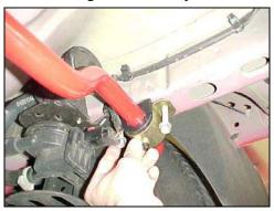
6.) Now its time for the Hotchkis end link installation. See pictures below. Make sure to place the appropriate washer before each nut. It's a good idea to lube the end link bushings with the provided grease. Note: for street use, use the hole closest to the end of the bar
