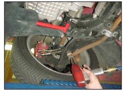
3.) Now remove the sway bar mounts but keep the brackets near by because you will use them again. The remove the bar.
