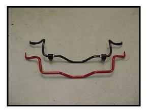
10) Re-install your new Hotchkis sway bar in the same manner as the stock sway bar removal. Install using the included Hotchkis polyurethane bushings and brackets. It's a good idea to install the bushings and brackets after the bar is in position. Lube the inside of each bushing with the provided grease. Use bushing prt # 5339.
