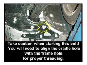
2 – Install the front cradle nuts and torque to **116 ft-lbs**.
