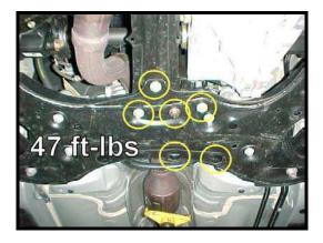
5 – Install the 4 nuts to secure the steering rack to the cradle. Torque to 45 ft-lbs.
