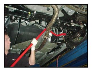
7) Lube the inside hole of your new Hotchkis polyurethane bushings and install the bushings on to the bar.
