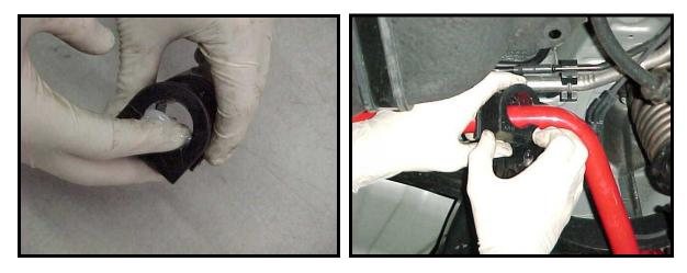
8) Place the provided bushing bracket over the bushing and set the sway bar into it's proper position. Install the provided nut and bolt & flat cut washer to secure the bracket to the frame of the vehicle.
