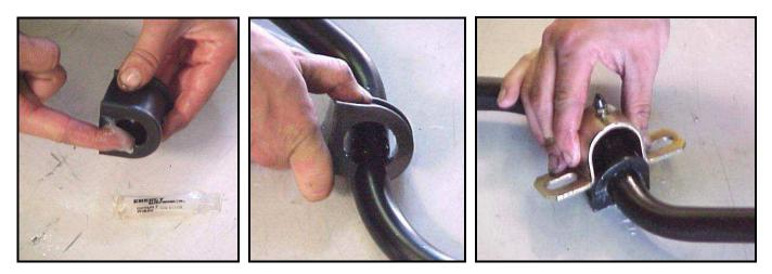
4) Use the grease provided to apply a heavy coat of grease to the sides of the bushings on the "dog bone" end links. Attach the mounting brackets to the end links using hardware kit #T1712. Attach the other end of the links to the sway bar. Leave the attaching hardware loose.
