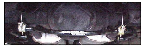
**<u>IMPORTANT</u>**: For maintenance, use the zerk fittings to grease the bushings at least once a year (15,000 miles) or when excessive noise occurs. <u>Use a non-lithium based grease only</u>! A lithium-based grease can wash out with water and should not be used.
