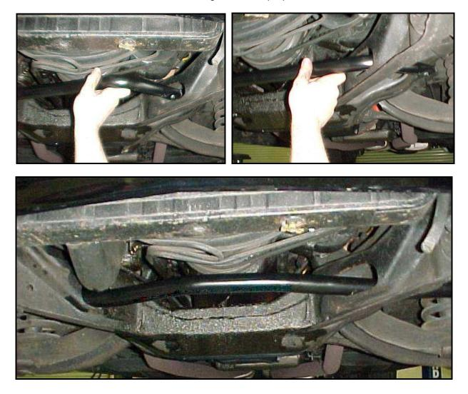
8) Use the grease pack provided to put a heavy coat of grease on the inside of the sway bar bushings. Place the bushings over the bar with the cut in the bushing towards the rear of the vehicle. Push the bushing retainer brackets into place on the bar and bolt them into place <u>using</u> the stock mounting hardware in the front holes only. **Do not** tighten the stock hardware.
