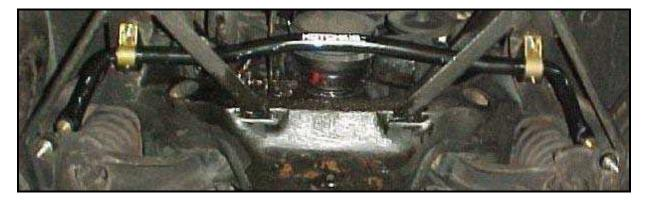
**IMPORTANT:** For maintenance, use the zerk fittings to grease the bushings at least once a year (15,000 miles) or when excessive noise occurs. <u>Use a non-lithium based grease only</u>! A lithium-based grease can wash out with water and should not be used.
