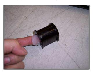
10) Open the bushing and push it over the bar. Make sure the flat side is facing down and the split is facing toward the front.
