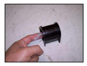
14) Open the bushing and push it over the bar. Make sure the flat side is facing up and the split is in the front.
