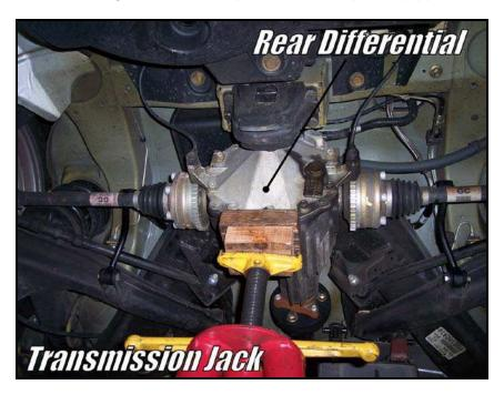
3) Remove the 4 bolts that secure the backside of the rear differential housing.
