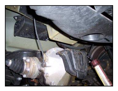
5) Next, detach the endlinks from the sway bar using a pair 13mm wrenches.
