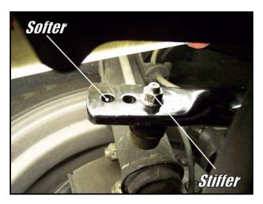
18) You are now finished with the Hotchkis front sway bar installation! Make sure that all hardware is fully tightened. On to the Hotchkis rear sway bar installation.
