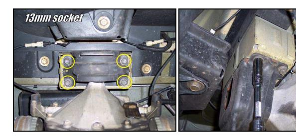
4) Slowly lower the transmission jack and let the differential and rear cradle frame tip downward.
