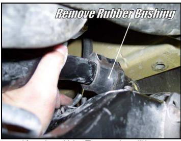
10) The bar can finally be removed from the vehicle. The sway bar will have to come out through the front, but it will take some patience to do so. Try to pull the passenger side end out first as shown in the picture. Once that end is free you can pull the bar completely out. Please note the orientation and position of the stock sway bar for reference for the Hotchkis sway bar.
