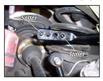
18) You are now finished with the Hotchkis rear sway bar installation! Make sure that all hardware is fully tightened before driving the vehicle.
