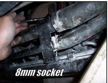
You will notice that the hard transmission lines lay on top of the coolant/transmission line bracket mounts. Make sure to move the transmission lines <u>below</u> the brackets. This will allow the bar to pass through between the coolant lines on top and the transmission lines on the bottom.
