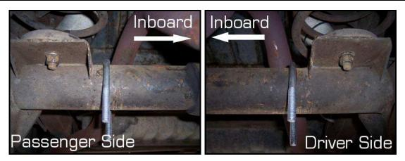
Next, apply the provided lube on the inside surface of the polyrethane bushings. Pop the bushings onto the sway bar. Slide the bushing brackets onto the bushings.
