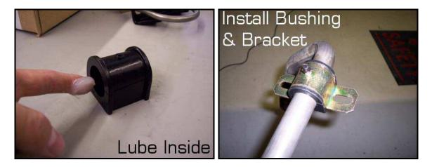
Apply a small amount of anti-seize to the threads of the U-bolts. Next position the axle bracket up against the axle tube. Raise the sway bar up to meet the axle bracket and allow the U-bolts to poke through the bushing bracket. Fasten the assembly together with the provided nut and washer. Do not fully tighten.
