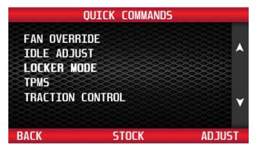
From the Quick Commands menu, use the buttons to the right of the screen to highlight Locker Mode.
