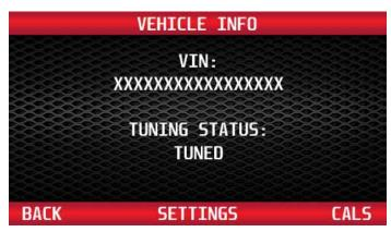
Select 'Settings' to view the current options that are programmed in the vehicle. Select 'Back' button to return to the previous menu. Use the buttons to the right of the screen to view all the settings programmed into the vehicle.
