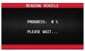
Once the programmer has completed the reading process, it will proceed to the Writing Vehicle mode. Continue to follow the messages on the screen. You may be prompted to turn the key to the 'Run' and 'Off' position during this process.
