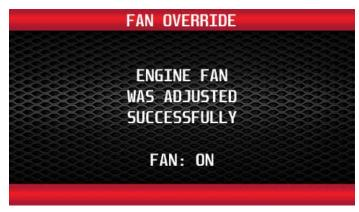
From the Quick Commands menu, use the buttons to the right of the screen to highlight Fan Override and press the 'On' button. This will manually override the engine fan cooling operation.
