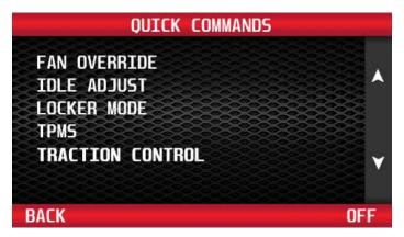
From the Quick Commands menu, use the buttons to the right of the screen to highlight Traction Control. Select 'Off' to turn off the factory traction control. These screens will then appear:
