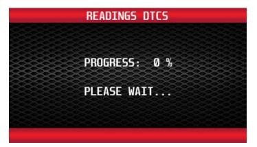
The programmer will immediately begin reading out the DTCs from the vehicle's computer. If no DTCs are present, the programmer will display the following message:
