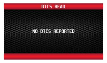
If the vehicle has any DTCs, the programmer will show the total number of DTCs reported from the vehicle's computer. Press 'Show' to see all the DTCs found.
