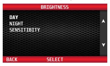
Use the buttons to the right of the screen to adjust the brightness of the display screen, from 1 to 9. Press the 'Back' button to return to the previous menu.
