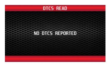
Prior to starting the programming process, the programmer will check for any Diagnostic Trouble Codes (DTCs). If any DTCs are present, the programmer will display them. You can review the DTCs before clearing.
