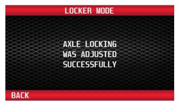
Select 'Adjust' to lock both the front and rear differentials. This will lock both front and rear below 20MPH. As you accelerate above 20MPH, the front disengages, above 30MPH, the rear disengages. When the vehicle speed drops below these thresholds, they automatically re-engage.
