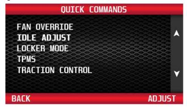
From the Quick Commands menu, use the buttons to the right of the screen to highlight Idle Adjust and press the 'Adjust' button.
