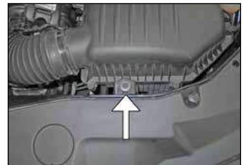
6. Remove the bolt that secures the air filter housing to the core support.
