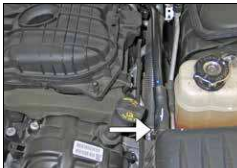
4. Disconnect the crank case vent hose from the air filter housing.
