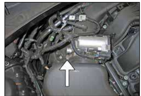
5. Loosen the hose clamp that secures the intake tube to the throttle body.
