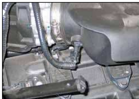
3. Disconnect the inlet air temperature sensor electrical connection.
