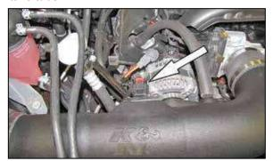
22. Reconnect the mass air sensor electrical connection.
