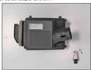
16. Remove the mass air sensor from the factory air box.
