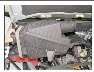
6. Pull up the air box to release it from the mounting grommets and then remove the factory air box from the vehicle.
