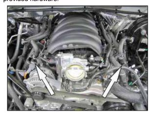
12. Remove the two factory crank case vent tubes from the vehicle.
