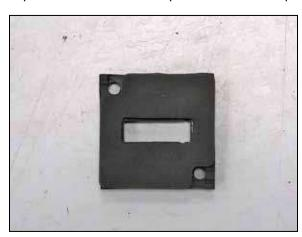
15. Install the provided gasket onto the K&N® mass air sensor adapter as shown.
