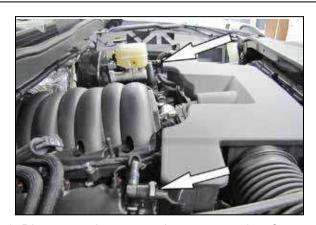
3. Disconnect the two crank case vent tubes from the intake plenum.
