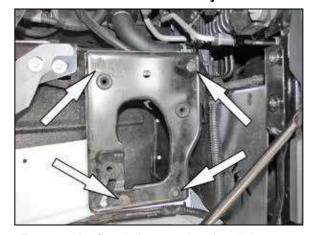
7. Remove the four bolts securing the air box mounting tray and then remove the tray from the vehicle.
