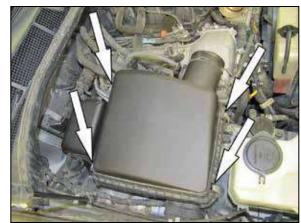
6. Release the four clips retaining the upper air filter housing and then lift off the housing and remove the factory air filter.
