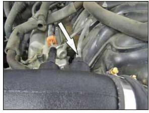
12. Connect the fuel pressure regulator vent hose to the fitting installed into the K&N® intake tube.
