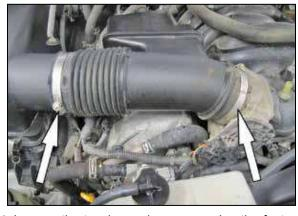
4. Loosen the two hose clamps securing the factory intake tube
