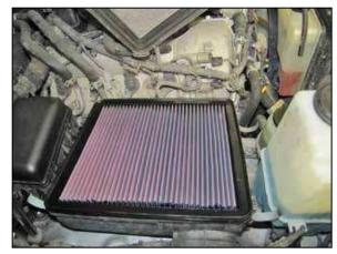
7. Install the K&N® air filter into the lower air filter housing and replace the upper housing but do not latch the retaining clips at this time.
