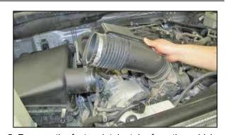
5. Remove the factory intake tube from the vehicle. NOTE: K&N Engineering, Inc., recommends that customers do not discard factory air intake.
