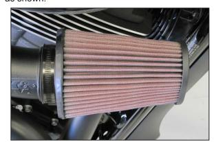
9. Install the K&N® air filter and secure with the provided hose clamp.
