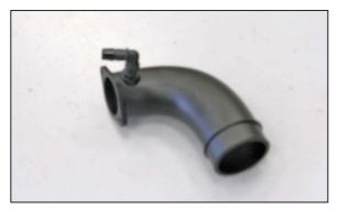
7. Install the provided 90° fitting into the K&N® throttle body adapter tube as shown.
