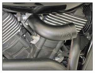
8. Connect the factory crank case breather hose to the fitting installed into the K&N® throttle body adapter tube. Using the factory hardware and gasket, secure the throttle body to the throttle body as shown.
