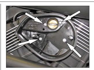
4. Remove the two throttle body bolts and the two filter back plate mounting bolts shown.
