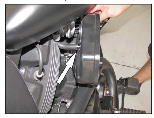
5. Pull the filter back plate away so that the crank case breather hose connection can be accessed. Release the spring clamp and then disconnect the crank case breather and remove the back plate from the vehicle.
