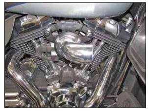
10. Install the two remaining O-Rings and K&N® breather bolts into the tube adapter. Tighten all of the hardware at this time.
