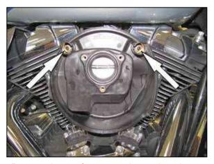
5. Remove the two factory crank case breather bolts and then remove the filter back plate from the vehicle.
