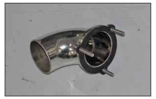
6. Install the three provided tube mounting bolts into the K&N® intake tube and then install one of the two provided gaskets onto the bolts.
