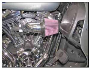
11. Install the K&N® air filter and secure with the provided hose clamp.
