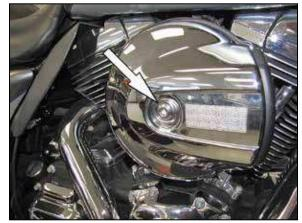
3. Remove the bolt securing the air filter cover and then remove the cover from the vehicle.
