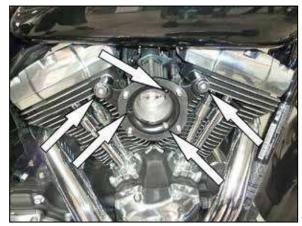
10. Using the two provided crankcase breather bolts; install the back plate onto the vehicle. Do not tighten bolts at this time. Install the provided gasket between the throttle body and back plate and then secure with provided hardware.
