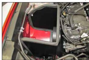
12. Install the heat shield assembly into the vehicle and secure with the factory coolant reservoir nut and air box mounting nut.
