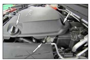
3. Remove the oil fill cap and loosen the hose clamp securing the intake hose to the throttle body. Remove the bolt securing the intake plenum to the engine.
