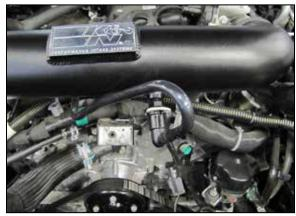
19. Rotate the crank case vent line and fitting so it alians with the quick connect fitting and then connect.
