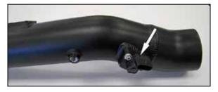
13. Remove the mass air sensor from the factory air filter housing and install the sensor into the K&N® intake tube using the provided hardware.
