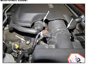
2. Loosen the hose clamp that secures the intake hose to the air filter housing. Using a screwdriver, unlock the small clamp that secures the vent line to the connector and then disconnect the vent line. Remove the bolt securing the intake plenum to the
