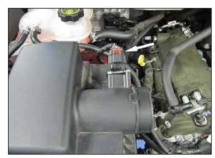
5. Release the red locking tab and then disconnect the mass air sensor electrical connection and unhook the harness from the air filter housing.
