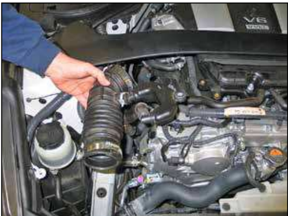
8. Remove the right side intake hose from the vehicle. NOTE: It will be necessary to release the spring clamp which secures the crank case vent hose to the valve cover port and then disconnect the crank case vent hose from the valve cover.
