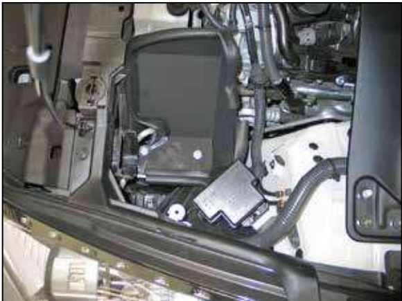
18. Install the heat shield assembly into the vehicle so that the mounting pins engage into the air box mounting grommets.
