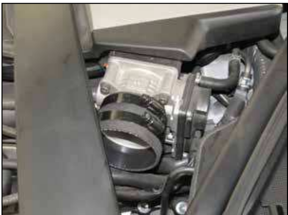
14. Install the coupling hose (084036) onto the driver's side throttle body and secure with the provided hose clamp.
