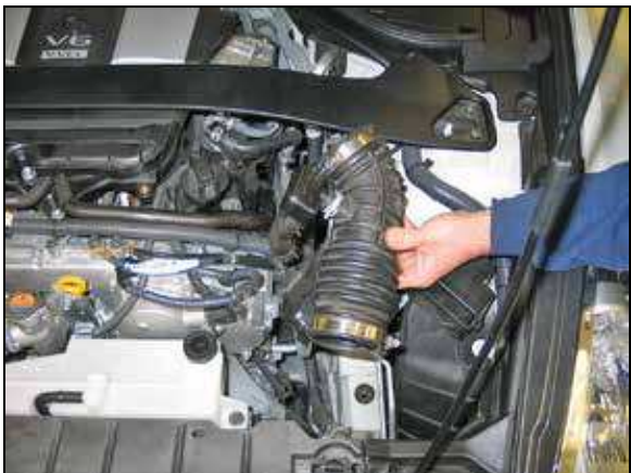
13. Remove the driver's side intake hose from the vehicle. NOTE: It will be necessary to release the spring clamp which secures the crank case vent hose to the valve cover port and then disconnect the crank case vent hose from the valve cover.
