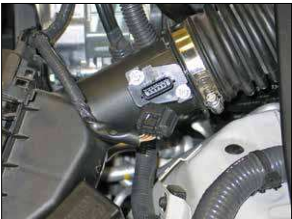
9. Disconnect the Driver's side mass air sensor and unhook the wiring harness from the air box.
