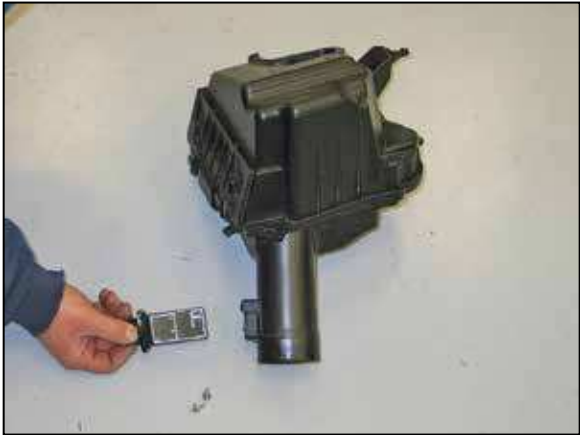
20. Remove the two screws securing the mass air sensor to the driver's side air box and then remove the mass air sensor from the air box.
