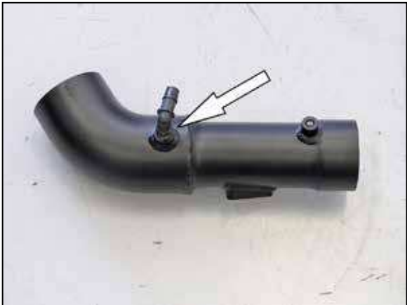
19. Install the provided 90° NPT vent fitting into the driver's side K&N® intake tube (27466) as shown. NOTE: Plastic NPT fittings are easy to cross thread. Install the vent fitting "hand" tight, then turn it two complete turns with a wrench.
