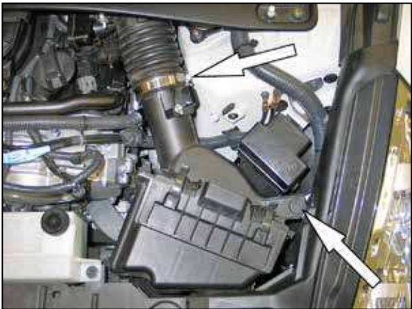
10. Loosen the hose clamp which secures the right side intake hose to the air box. Remove the bolt which secures the air box to the inner fender.
