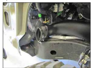
43. Install the provided coupler hose (08711) onto the lower tube and secure with the provided hose clamp.
