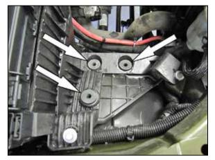
20. Install the provided insert nuts into the air filter housing mounting grommet locations.
