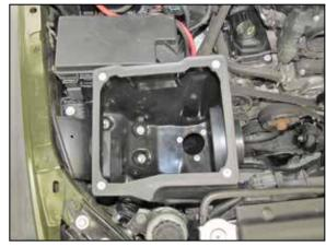
25. Install the air filter housing assembly into the vehicle onto the insert nuts and secure with the provided hardware.
