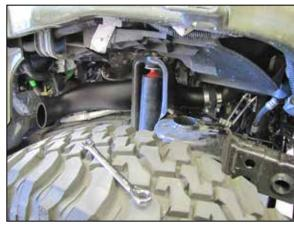
40. Install the lower tube into the coupler and align the mounting bracket with the nut extension. Secure the tube with the provided hose clamp and hardware.
