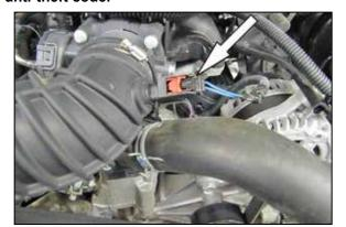
2. Release the red locking tap and then disconnect the inlet air temperature sensor electrical connection.
