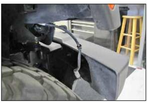
14. Remove the marker light bulb from the housing and disconnect the harness retaining clip from the fender.
