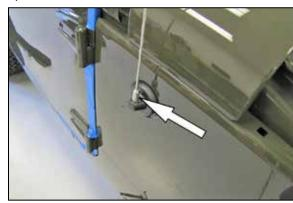
8. Remove the antenna mast.
