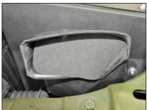
59. Use the provided dense foam to plug the fresh air intake duct when using in extreme wet
