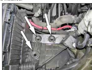
19. Remove the three air filter housing mounting grommets shown.
