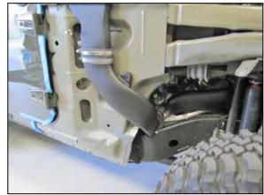
44. Install the provided coupler hose (08698) onto the corner tube, and then install the Corner tube assembly as shown, snug the hose clamps but leave them loose enough to provide adjustment.
