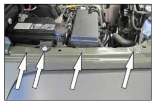
16. Remove the four bolts securing the top of the fender to the inner structure.
