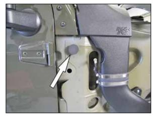
54. Peal the backing of the provided damper pad and then install it as shown on the inner body.
