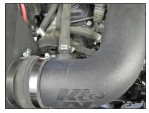
35. Connect the crank case vent hose as shown and secure with the provided hose clamp.
