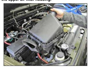
5. Lift up the air filter housing to dislodge it from the mounting grommets and then remove it from the vehicle.
