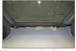
6. On vehicles equipped with rock sliders or running boards, remove the passenger side to gain access to the lower fender mounting bolts.
