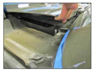
41. Install the snorkel mounting bracket (073219) onto the factory fender mounting points on the cowl using the provided hardware.
