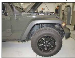
55. Reinstall the fender and secure with the factory hardware. Then reconnect the marker light and install the antenna mast.
