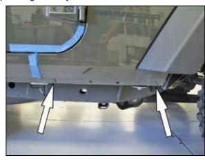
13. Remove the two lower fender bolts.
