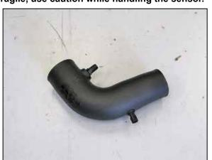
33. Remove the O-ring from the sensor and then install the sensor into the grommet installed into the  $K\&N^{\odot}$  intake tube.
