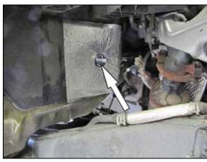
37. Install the provided nut extension and fender washer onto the stud as shown.
