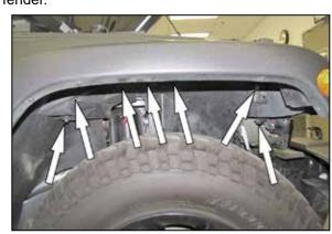
15. Remove the seven inner fender bolts.
