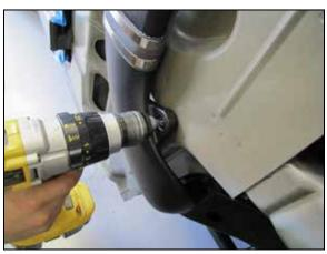
51. Adjust the corner tube and secure the hose clamps. Using the mounting hole in the corner tube as a guide, drill a 5/64" id hole into the inner body panel.
