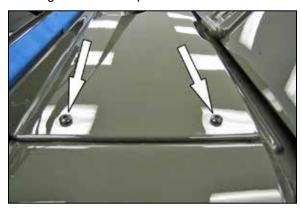
10. Using the T30 socket, remove the two bolts securing the cowl panel to the right side fender.
