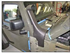
42. Temporarily install the snorkel and secure with the factory cowl bolts.
