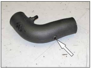
31. Install the provided grommet into the K&N<sup>®</sup> intake tube as shown.
