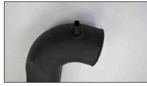
13. Remove the inlet air temp sensor from the factory inlet tube. Then remove the "O" ring from the sensor. Install the provided grommet onto the K&N<sup>®</sup> intake tube. Then install the inlet air temp sensor into the grommet.
