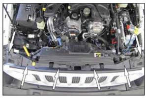
6. Remove the 6 clips at the top of the grill that secure grill to core support.
