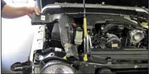
8. Remove the two bolts that secure the inlet scoop to the core support and remove inlet scoop.
