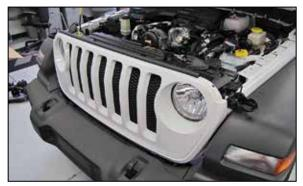
10. Reinstall the grill reengaging the lower clips one at a time then reinstall the six clips that hold the grill to the top of the core support. 15. Install the K&N<sup>®</sup> intake tube assembly onto the K&N<sup>®</sup> airbox with provided hardware. Note the orientation of the K&N<sup>®</sup> intake tube.
