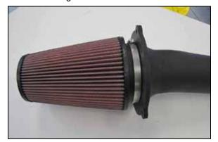
14. Install the K&N $^{\rm \tiny B}$  air filter onto the K&N $^{\rm \tiny B}$  intake tube.
