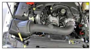
17. Install the K&N<sup>®</sup> intake assembly into the hose at throttle body first, then engage the K&N<sup>®</sup> airbox mounts into the factory airbox mounting location. Secure K&N<sup>®</sup> intake assembly with provided clamp.
