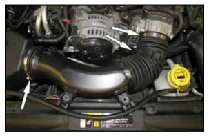
4. Loosen the two hose clamps that secure the intake tube and disconnect the inlet air temperature sensor electrical connection. Remove the factory intake tube from the vehicle.
