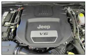
2. Lift up the engine cover to dislodge it from the mounting studs and then remove the cover from the engine.
