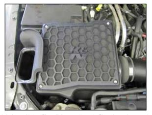
22. Install the filter lid onto the air filter housing and secure with the provided hardware. NOTE: A foam insert has been provided to use in the fresh air intake duct during extreme conditions.
