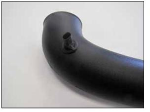
14. Remove the inlet air temperature sensor from the factory intake tube. Using the provided grommet install the inlet air temperature sensor into the K&N<sup>®</sup> intake tube.
