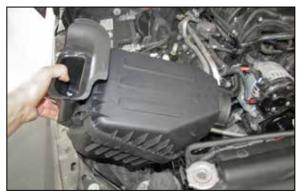
6. Remove the factory air filter housing from the vehicle.
