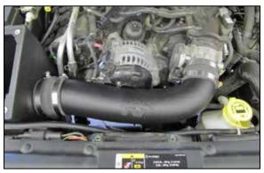
16. Install the provided hump coupler (08699) onto the K&N<sup>®</sup> intake tube and then install the assembly into the vehicle. Adjust the tube for best fit and then secure with the provided hose clamps. Reconnect the inlet air temperature sensor electrical connection. 21. Assemble the three parts of the filter lid.
