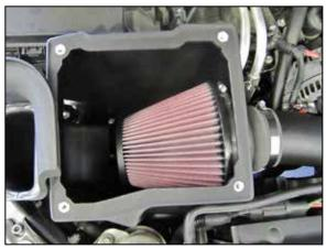
20. Install the K&N<sup>®</sup> air filter onto the adapter and secure with the provided hose clamp.
