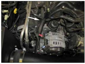
17. Install the provided crank case vent line onto the fitting installed into the intake tube and onto the factory hardline.
