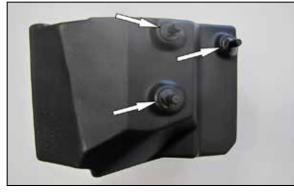
7. Install the three mounting studs provided onto the K&N $^{\odot}$  air filter housing using the provided hardware.
