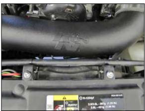
19. Install the "L" brackets onto the fan shroud using the provided hardware and then secure the coolant hose with the tie wraps.
