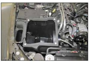
12. Install the K&N<sup>®</sup> air filter housing into the vehicle so the mounting studs insert into the factory mounting brackets.
