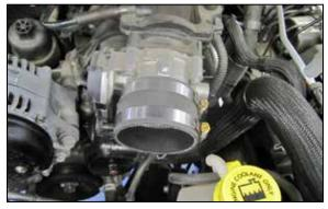
13. Install the provided coupler (08690) onto the throttle body and secure with the provided hose clamp.
