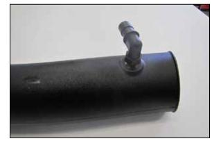
15. Install the provided 90° fitting into the K&N®
