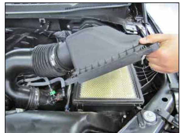
5. Lift up and remove the upper air filter housing and factory air filter.
