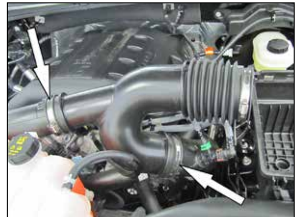
6. Loosen the hose clamps securing the intake tube to the two turbo inlet tubes and then remove the intake tube from the vehicle. NOTE: K&N Engineering, Inc., recommends that customers do not discard factory air intake.
