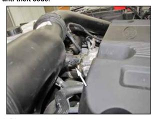
2. Disconnect the inlet air temperature sensor.
