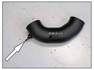
10. Install the provided vent fitting into the K&N<sup>®</sup> intake tube as shown.
