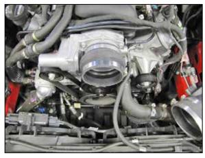
9. Install the provided hump coupler hose (08418) onto the throttle body and secure with the provided have alarm
