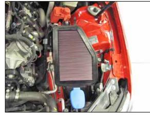
7. Replace the air filter with the provided K&N<sup>®</sup> performance air filter and reinstall the upper air box assembly. Secure the upper air box assembly with the five factory retaining clips.
