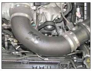
11. Install the K&N<sup>®</sup> intake tube into the coupling hose at the mass air sensor and then into the hose at the throttle body. Adjust the tube for proper fit and then secure with the provided hose clamps.
