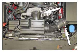
5. Loosen the hose clamps securing the intake plenum to the throttle body and to the mass air sensor then remove the plenum from the vehicle. **NOTE: K&N Engineering, Inc., recommends that customers do not discard factory air intake.**
