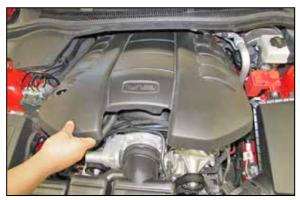
2. Remove the oil fill cap and then remove the decorative engine cover. Reinstall the oil cap to prevent debris from entering the engine.
