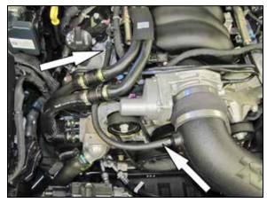
12. Connect the provided crank case vent hose to the fitting installed into the  $K\&N^{\otimes}$  intake tube and then connect the open end to the port on the valve cover.
