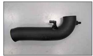
6. Install the provided 90° and straight vent fittings into the K&N $^{\! \rm B}$  intake tube as shown.
