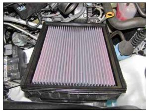
6. Install the K&N® air filter into the lower air filter housing and then reinstall the upper housing. Do not secure the lid at this time.
