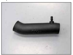
9. Install the provided NPT vent fitting into the K&N® intake tube as shown.
