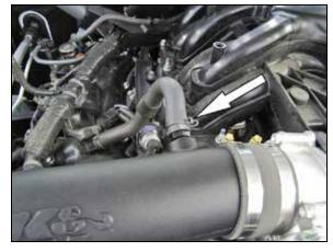
11. Connect the factory crank case vent hose to the fitting installed into the K&N® intake tube and secure with the factory spring clamp.
