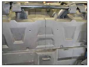
12. Reinstall six of the eight bolts removed in step #3. Reinstall the seats.
