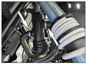
6. Release the clamps that secure the BOV hose and crank case vent hose to the intake tube and then disconnect the hoses from the tube.
