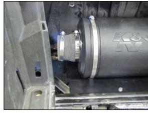
18. Install the provided coupler hose (084055) onto the filter adapter and secure with the provided hose clamp.
