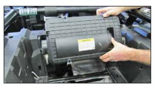
5. Loosen and remove the two hose clamps that secure the fresh air and clean air ducts to the air filter housing. Remove the air filter housing from the vehicle.
