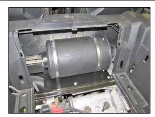
17. Install the filter canister assembly onto the mounting tray and connect the fresh air inlet hose. Adjust the canister and hose for best fit and then secure the canister and hose with the hose clamps. NOTE: Due to differences in the production factory foil heat shield, the heat shield may need to be reformed to allow the canister and
