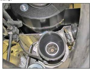
19. Install the provided coupler hose (08667) onto the turbo inlet and secure with the provided hose clamp.
