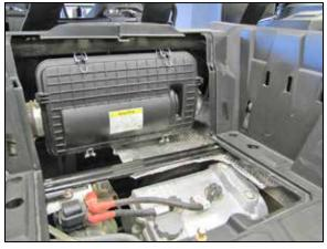
4. Release and lift off the engine cover.
