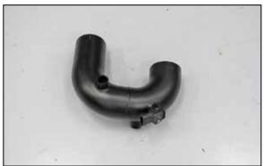
21. Install the inlet temperature sensor into the K&N® intake tube and secure with the provided hardware.
