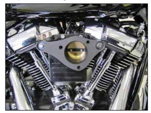
8. Using the provided throttle body mounting bolts, install the base plate onto the engine. Do not completely tighten the bolts; they are just being used to hold the base plate in the correct position at this time. Secure the servo cover to the back of the base plate with the hardware provided. Now install the remaining breather O-rings into the base plate and secure the base plate with the provided breather bolts. Then remove the three throttle body
