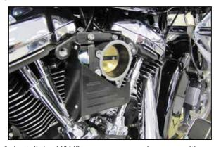
6. Install the K&N® servo cover and secure with the provided hardware to the original servo cover mounting bolt locations.
