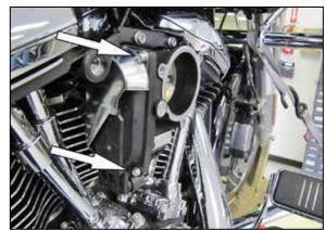
5. Remove the two servo cover bolts shown.
