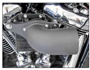
10. Install the intake tube onto the base plate. NOTE: Apply one drop of the provided thread locker to the threads of each bolt.
