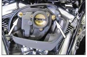
4. Remove the two breather bolts shown and then remove the rear air filter housing from the vehicle. NOTE: K&N Engineering, Inc., recommends that customers do not discard factory air intake.
