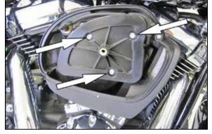
3. Remove the three bolts that secure the air filter element and then remove the air filter and crank case breather tubes.
