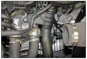
14. Remove the bypass hose retaining clip shown and flip it to the other side of the bracket and reinstall, then reinstall the bypass hose into the clip.
