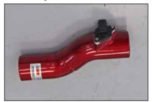
13. Install the mass air sensor into the K&N<sup>®</sup> intake tube and secure using the provided hardware.
