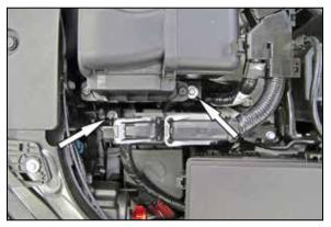
Remove the two bolts that secure the factory air filter housing to the inner fender and then remove the complete intake assembly from the vehicle. NOTE: K&N Engineering, Inc., recommends that customers do not discard factory air intake.
