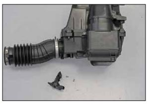
12. Remove the mass air sensor from the factory air filter housing.
