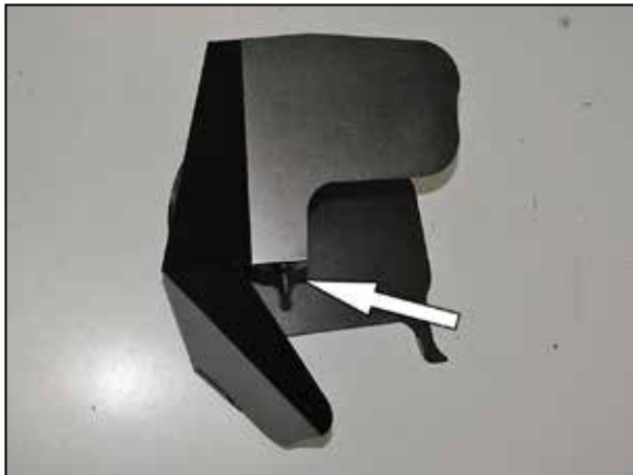
9. Install the mounting stud onto the heat shield using the provided hardware.
