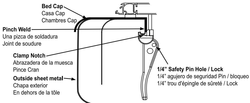
If traveling with the Tonneau in the folded position it is recommended to use a safety pin or lock in the front clamps.
