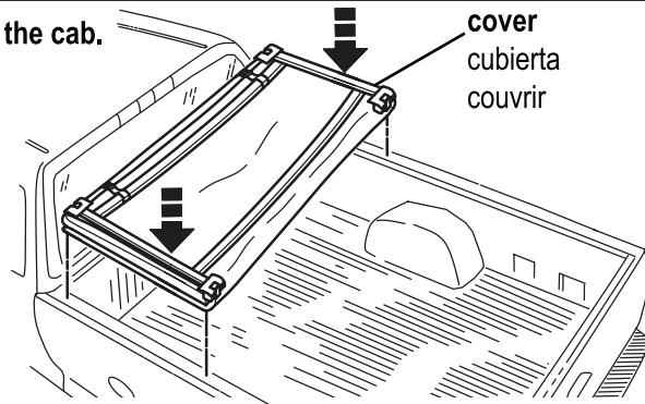
**If a gap exists between the cover and the bulkhead of the truck proceed to step 3 and or 4. If not proceed to step 5.**
