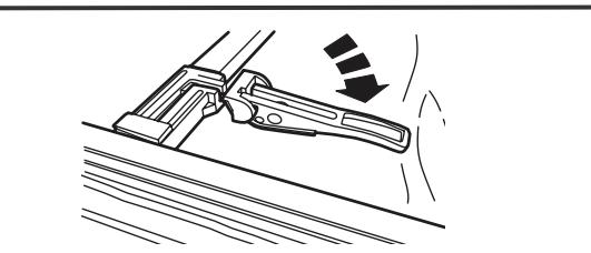
**When stowing cover, position all clamps in their storage positions or latch handles may puncture cover and void warranty.**
