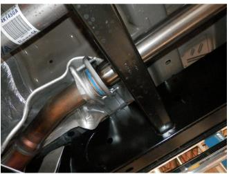
**Step 3.** Your new MAGNAFLOW system comes with two inlet pipe assemblies. The assembly that has the flange welded to it is for year spread 2015 - 2020. The pipe without the flange will use the slip flange in the hardware kit and is for years 2021. Loosely attach the correct pipe assembly for your year of vehicle using either the OE hardware or the supplied hardware.
