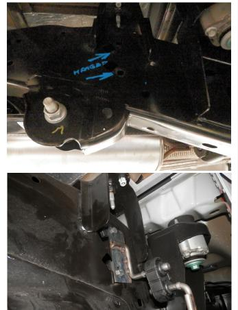
**Step 5.** Locate the two square holes in the passengers side of the vehicles subframe. Attach the two supplied U-Type panel nuts as shown in the diagram. Losely bolt the supplied Hanger Bracket Assembly to the panel nuts using the supplied bolts.
