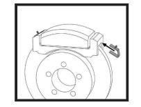
Slide the stainless steel clips on each side of the brake caliper bracket. Fit should be snug and secure.
