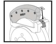
Place the cover over the caliper and position hole in bridge over the threaded stud and onto the clip (may require some force to pull second hole over stud).
