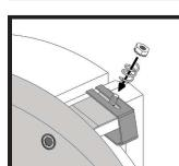
Install the supplied locknuts onto the threaded studs to secure clip to bridge. Tighten with 3/8-inch wrench or socket to 25 inch pounds (about 1/4 turn past finger-tight). Do not over tighten.
