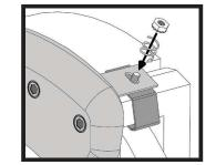
Install the supplied locknuts onto the threaded studs to secure bridge to clip. Tighten with 3/8-inch wrench or socket to 25 inch-pounds (about 1/4 turn past finger-tight). Do not over tighten.
