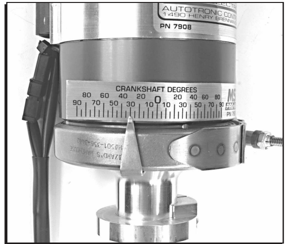
Figure 6 Applying the Timing Tape.
