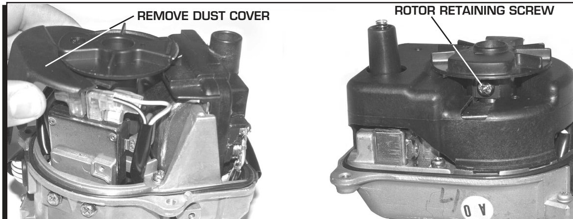
Figure 4 Replacing the Rotor.
