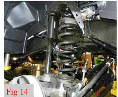
18. It is necessary to trim the tab off the coil spring isolator for re-install. Use a cutting tool and remove the tab.
