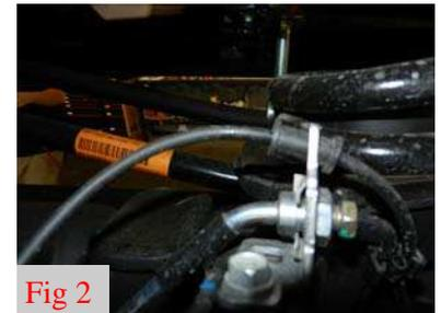
4. Locate the 2 brake line/ABS brackets attached to the axle and remove brackets.
