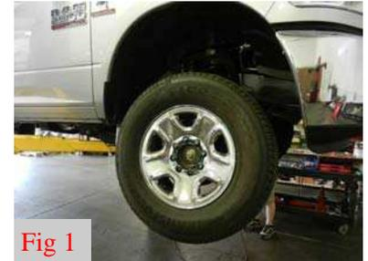
2. Record stock vehicle ride height measurements on both the front and the rear, this will provide a guideline on vehicle rake and lift height. Measure from the center of the wheel up to the bottom edge of the fender well opening and record on chart provided on page 2.
