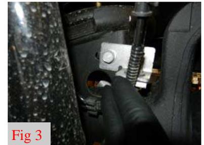
5. Locate the brake line/ABS bracket on the inside of the frame rails and remove.
