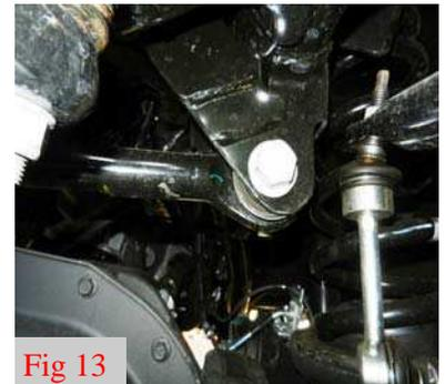
17. Lower the axle enough to remove the front springs. Make sure to not over extend the brake/ABS lines.
