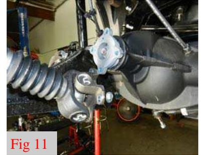
14. With the axle fully supported, remove the lower shock bolts.
