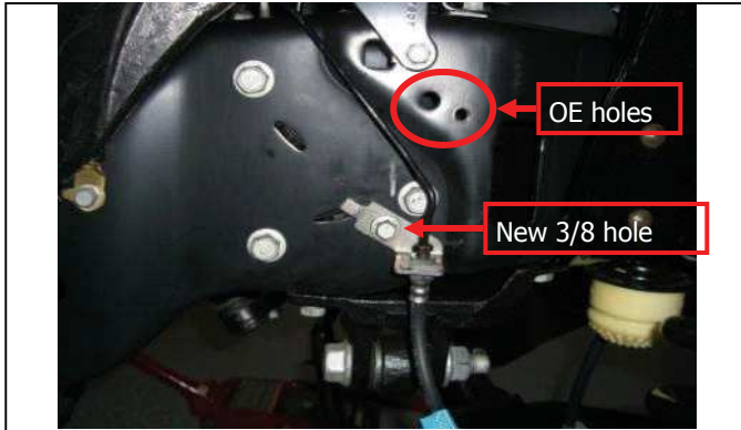
Shown dr. side new 3/8 brake line hole location.
