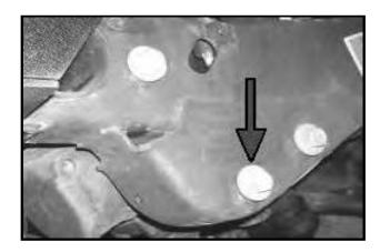
4. Place skid plate in location to line up with the lower bumper mount and the lower side frame mount.
