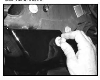
5. Secure to bumper and frame using hardware removed in steps 2 & 3.
