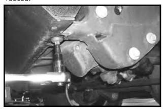
3. Remove the lower steering box mounting bolt DO NOT DISCARD. Hardware to be reused.
