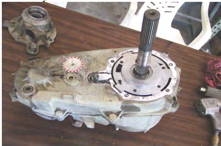
Photo 1. NP231 after completion of the first four steps of the disassembly process. The oil pump pickup tube may need to be removed before the case halves can be split
