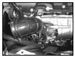
Step 12 Loosen the hose clamp securing the intake elbow to the throttle body so it can be rotated.
