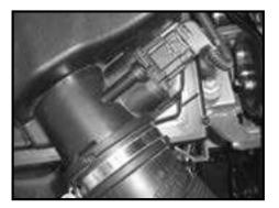
Step 2 Release locking tab and disconnect the mass air flow sensor electrical connector.
