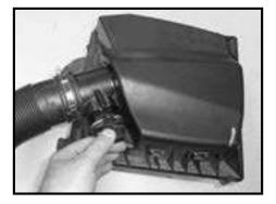
Step 8 Remove the two screws securing the mass air flow sensor in the factory airbox and then remove the mass air flow sensor from the airbox.
