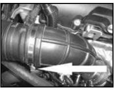
Step 3 Loosen the hose clamp securing stock intake tube to box.
