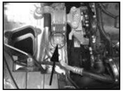
Step 5 Remove the front motor mount bolt. Note: Bolt will be reused in later step.
