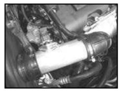
Step 15 Connect the mass air flow sensor connector.
