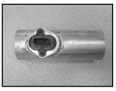
Step 9 Install mass air flow sensor into the Spectre Intake and secure with provided hardware.
