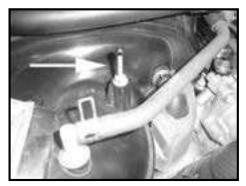
Step 14 (Trucks with 5.7L Engines) Remove the front engine cover mounting stud from the intake manifold.
