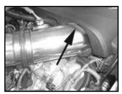
Step 13 (Trucks with 4.6L Engines) Install the factory engine cover. You may have to trim the engine cover slightly so that it does not interfere with the new intake tube.
