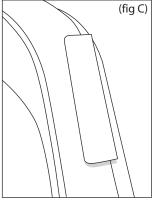
Remove the red backing from the adhesive. Insert the vertical leading edge of the sidewind into the channel behind the mirror assembly. (fig 1) Insure the adhesive strip on the tab on the bottom of the sidewind is securely fastened to the **OUTSIDE** of the flexible weatherstripping. (fig 2)
