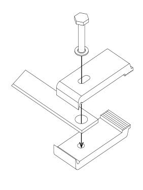
3) With the bolt head facing the logo, place the support bar underneath the rear flap. Close the flap and secure.
